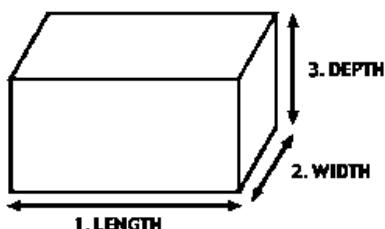
Box measurements always correspond to the inner dimensions of the box unless otherwise specified. This is done to ensure a snug and protective fit around your product. The size of your contents actually determines the inner box dimensions. Simply measure the Length (L) x Width (W) x Depth (D) (or height).
